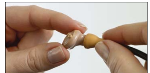
3c. If you are listening to an In-The-Ear (ITE) style hearing aid, simply attach the listening tube to the sound outlet end.
