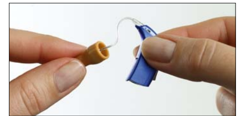
3b. If you are listening to a RITE hearing aid without mould, remove the dome and attach the listening tube directly to the sound outlet.
