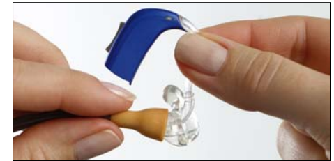
3a. Attach the listening tube to the earmould of the hearing aid.
